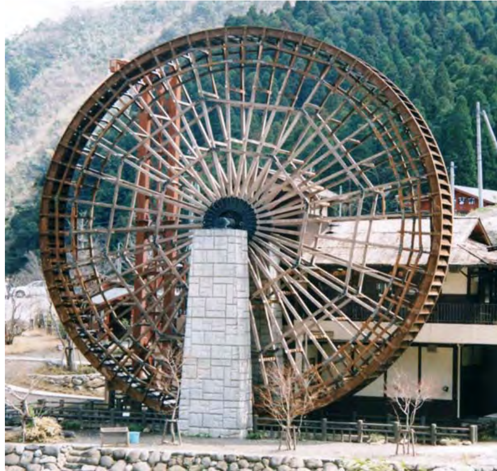
Back-pitch wheel for polishing rices & flour mill. 18m in dia. Built in 1993
