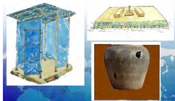
Option 7: HH dry toilet for outskirts, secondary farm, un-flooding, lack of water areas
