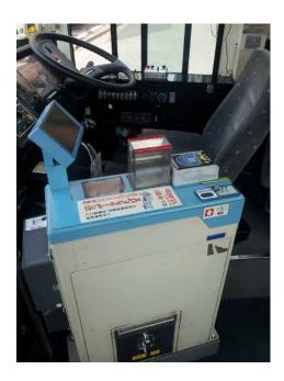
Fare box install beside the exit inside the bus to collect the fare, the driver collect the fare.
